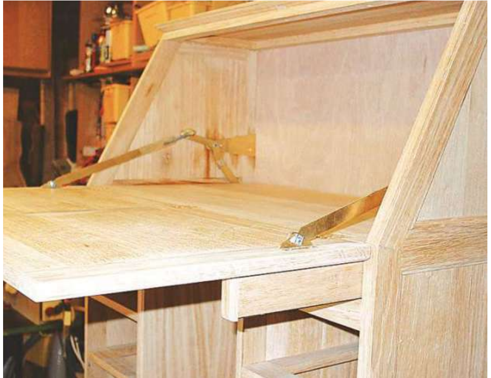
▲ Pic 13 Fit the desk flap and check that the lopers extend and retract smoothly
